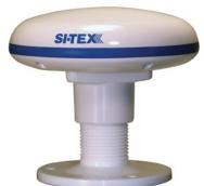
The professional-grade GPK-11 Max delivers accurate positioning data to any SI-TEX chartplotter or other navigation system requiring NMEA0183 GPS input. This highly sensitive, IP67 waterproof low-profile antenna can be pole or flush mounted and delivers better than three-meter accuracy for navigators, making it an ideal choice for a wide range of vessels from cruising yachts and commercial fishing boats to ocean-voyaging sailboats.
